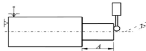
Fig. 5. Setup using a touch probe.
